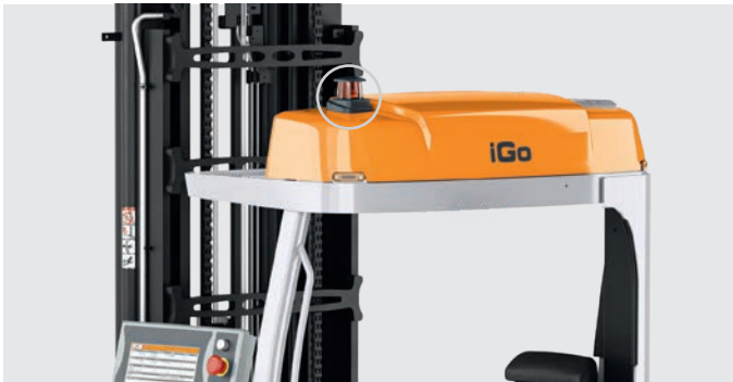
Maximum precision through navigation laser on the overhead guard
