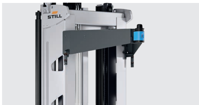
The sensitive navigation laser in the upper area of the truck enables maximum precision, efficiency and safety
