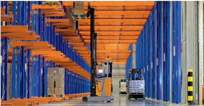
The FM-X iGo systems is equipped with a pallet positioning sensor for precise and efficient pallet handling even at the highest levels of the shelving
