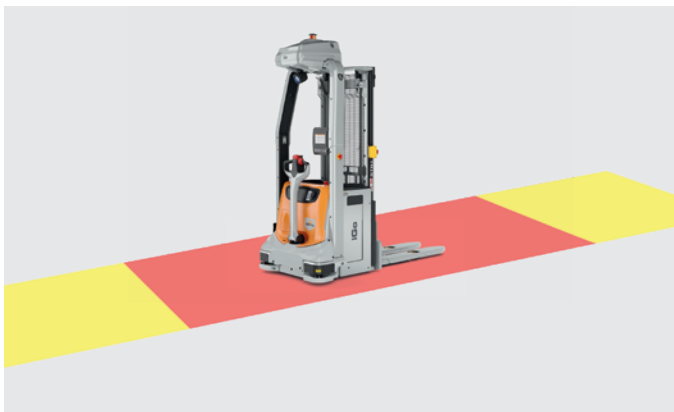
Dynamic safety fields around the truck ensure maximum safety and collision avoidance: Real-time adjustment of the driving speed depending on corner radius
